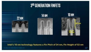
Putting a ruler on the fins, we come up with a fin width of 5-15nm, and ~7nm at half height. Gate width is ~110nm, compared with the ~85nm of the previous generation. Gate length is still an unknown, but we can speculate that it will be in the 18-20nm range, assuming dielectric thickness of ~8nm between the gate and contacts.
