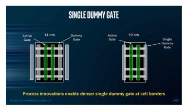
The dummy gates are shown in the plan-view image above, but what can't be seen is that he dummy gates usually overlap the end of the fin, unlike the left-hand schematic above. Here's a shot of 22nm PMOS gates on a fin:
