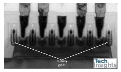
This clearly adds to the width of the cell, but it has the advantage of matching the performance of all the transistors on the fin. If we have a single dummy gate on the STI between the fins, as in the Samsung 14nm and earlier 20nm devices, then the source/drain cavity etch and the contacts are on or near the ends of the fin. They are then subject to overlay errors, increasing variation in both the contact resistance and the source/drain epi growth.
